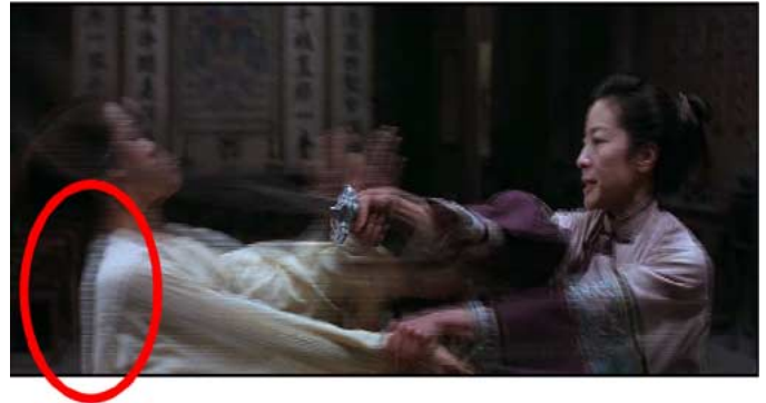
Fig. 1. Feathering effect appears while directly merging two fields in the motion area.
